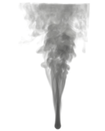
Fig. 18. Turbulent smoke plume driven by buoyancy.
